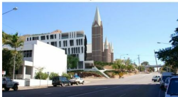
Figure SC6.3.4.5 Illustrates appropriate corner block front setback for development adjoining a heritage place. "A" and "B" is the street setback distance. The setback of new development is tapered to allow improved views to the heritage place.
